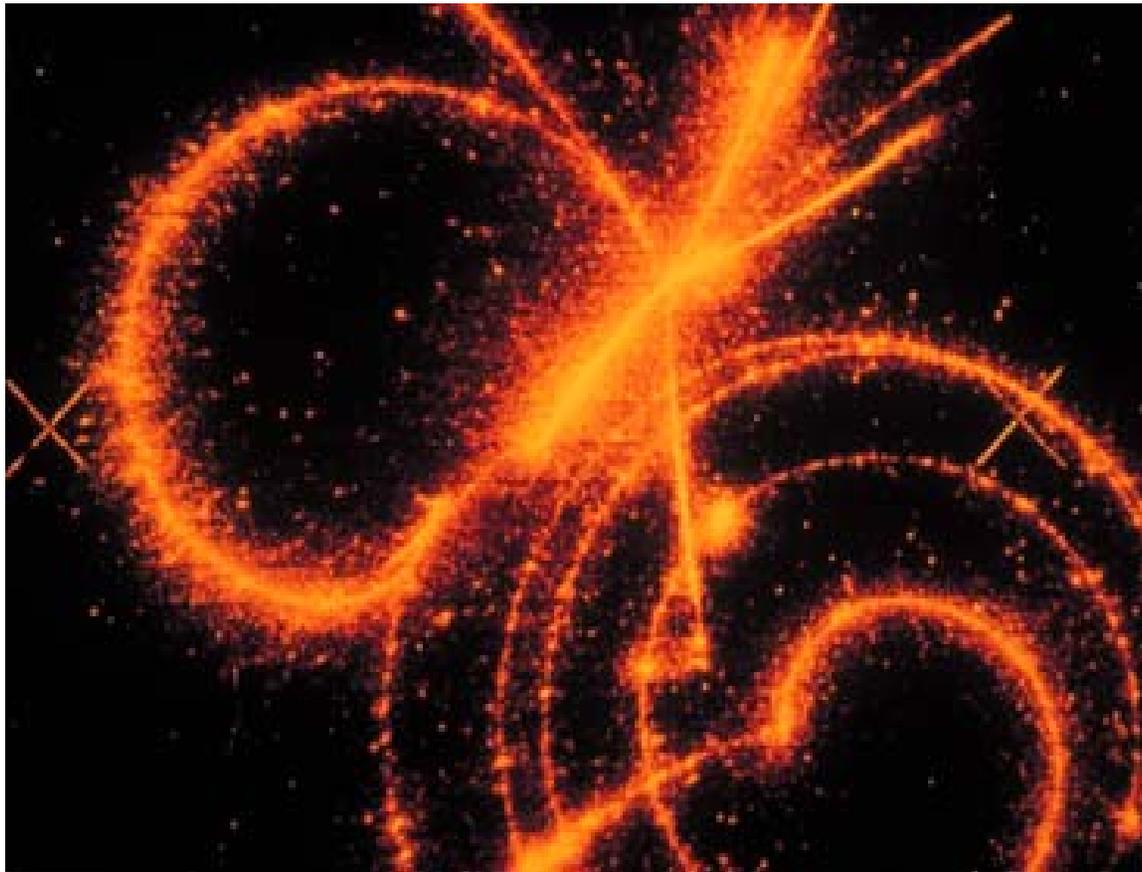
**Decay of positive pions captured on a streamer chamber image. CERN, 1990.**
