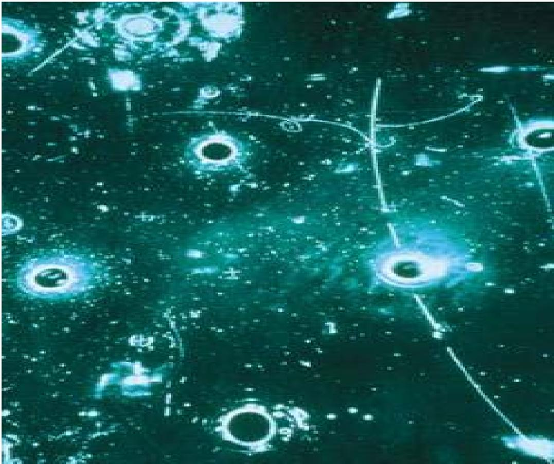
**A lepton event (a neutrino interacting with an electron and emerging as a neutrino);** the first observation of 'neutral currents' in the Gargamelle heavy liquid bubble chamber.
